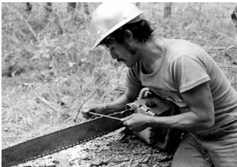
Figura 2. Afilado de cadena de motosierra (modelo Homelite 1050). Figure 2. Sharpening of the power saw chain (1050 Homelite model).
