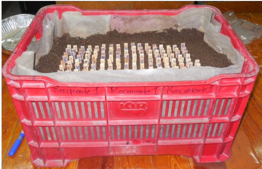
Figure 1. Test specimens exposed to the soil microcosm.
