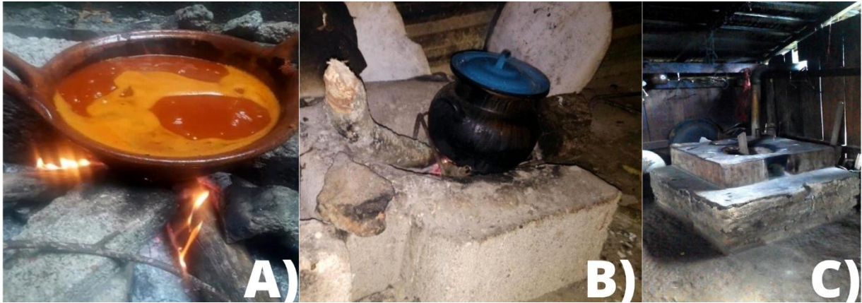
Figure 2. A) Open or three-stone brazier; B) Round or closed brazier; C) Wood-saving stove.
