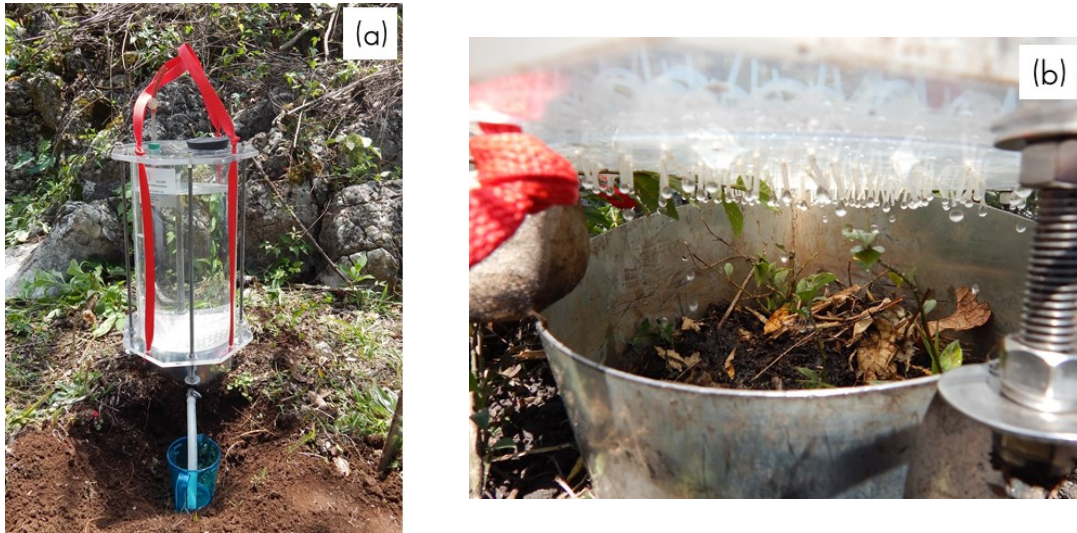
a) Infiltrimeter installed in the study site; b) Detail of the interior of a runoff measurement plot.
